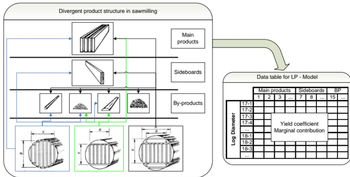
**Figure :** Different possible cutting patterns given a specific diameter
